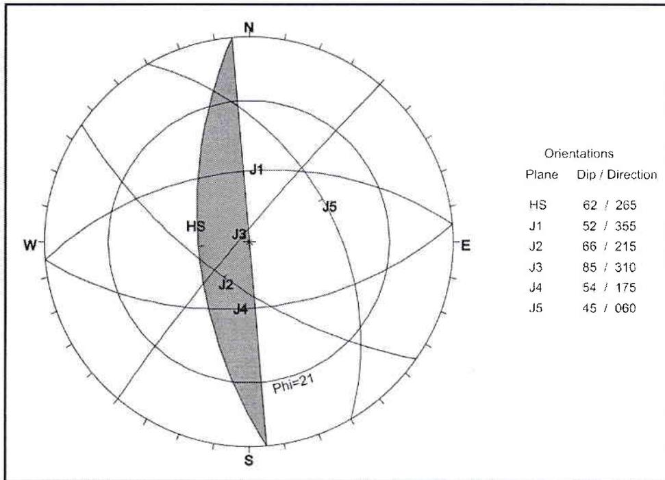
Figure 9: Slope stability analysis at the right bank of weir axis area.
